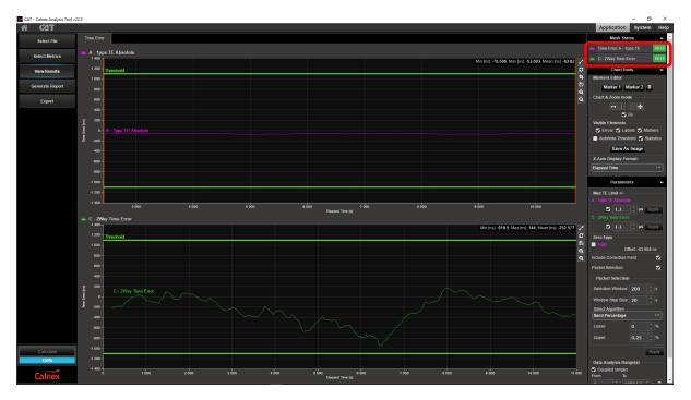
In this case the Max TE Limit +/- field can be set to 1.1us to give an automatic pass / fail indication. Using the same data the Max | pktSelected2WayTE | in this case is 918.5ns.
