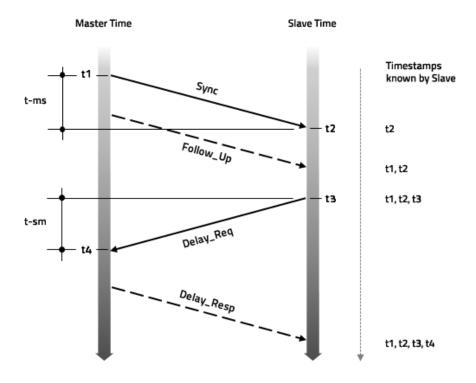
Once the Slave knows the timing of t1, t2, t3, and t4, it can calculate the mean propagation delay  $(T_{mpd})$  of the message path and slave clock offset. This can be calculated by:
