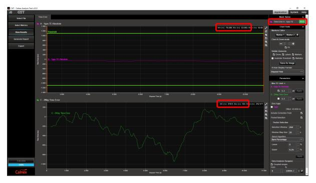
Maximising the 2Way Time Error graph allows the peak to peak value to be read from the Metric Statistics panel.
