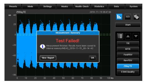
As Sentinel is displaying 2Way TE results for all the PTP messages rather than the pktSelected2WayTE result it is likely that the 2WayTE mask will fail. Further analysis in CAT is required to determine the peak to peak value of pktSelected2WayTE for APTS or the absolute magnitude for PTS. The 1PPS TE result can be read directly from the Sentinel measurement screen or in the measurement.summary.txt file.
