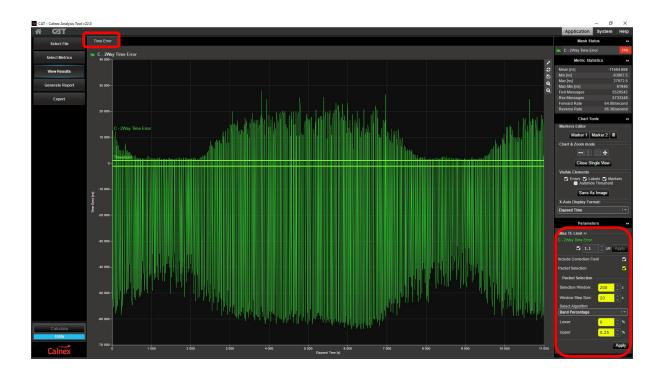
Press the Calculate button to display the pktSelected2WayTE results. Again the result can be compared against an absolute limit and the metric results are also displayed.
