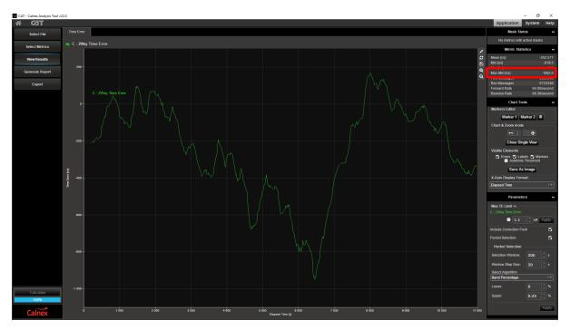
The 1PPS |TE| measurement is 76.506ns, well within the 1.35us limit while pktSelected2WayTE varies between -918.5ns and 144ns giving a peak to peak value of 1062.5ns which comes close to the 1100ns limit set by G.8271.2 and would require further investigation. The test should be run a second time with no GNSS connected to ensure that the 1PPS TE measurement remains within the 1.35us limit, while the T-TSC is in holdover.
