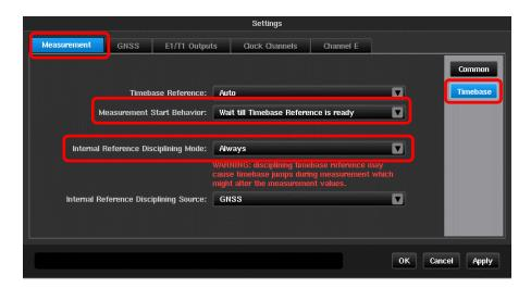
From a cold start, it takes around 15 minutes for the Sentinel internal Rubidium to warm up. With GNSS signal connected, the GNSS receiver needs to lock to at least 3 satellites before it can output a valid reference to the Rubidium for disciplining. The GNSS receiver will continue to output a valid reference while it is locked to at least three satellites.
