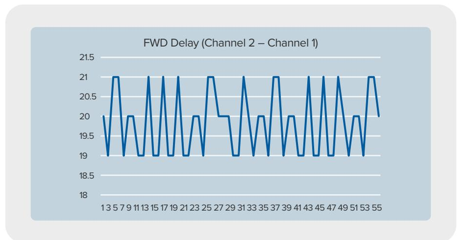
The results indicate a 20ns delay difference consistent with the 4m of added fiber.
